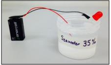
Electrolysis occurs when a stray electric current (our battery and wires) finds a path between two metals in the presence of an electrolyte such as salt water. As a result, the electrolyte begins to breakdown. Look closely at the wires in the water, one will have some bubbles!
